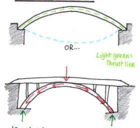
In order for an arch loridge to work it needs to have firm foundations, to allow all the members to push back against each other. The arch needs to be within a thrust line to stay nigid t supportive. This can be found by hanging a chain off the gap t then minoring it (light blue dotted line).
