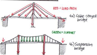
Suspension bridges allow for the longest spans. The bed of the bridge can be continuous, and is held up by cables stretched between piers. In the top bridge, these cables are rigid to directly connected to the longe deck. In the bottom longe, they hangvertically off another cable supported by the piers.
